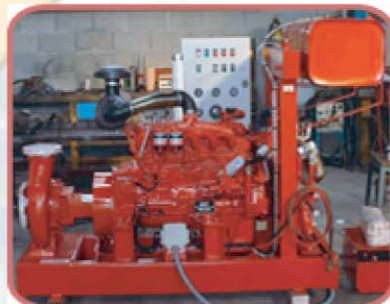
Skid motopompe 450 m 3 / h
